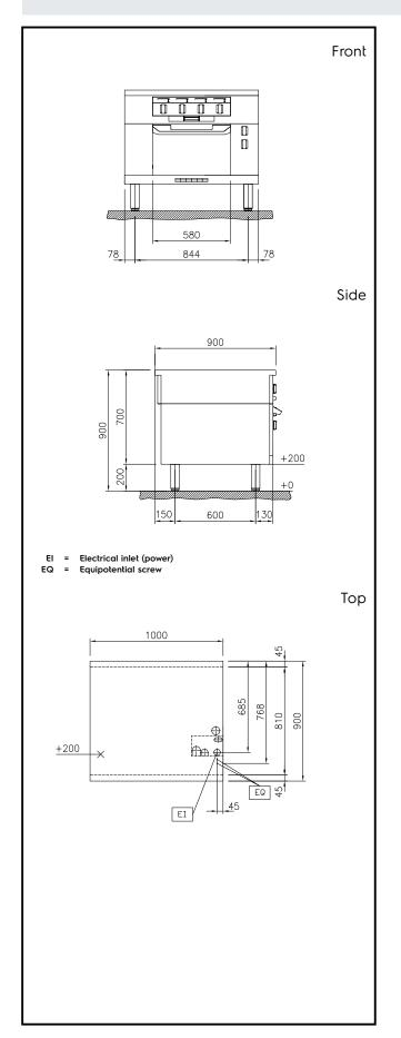
Modular Cooking Range Line thermaline 90 - Electric Free-cooking Top on Oven H=700
